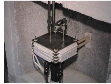
Fig. 2. Photograph of 4-cell stack using STS 430 as interconnects
